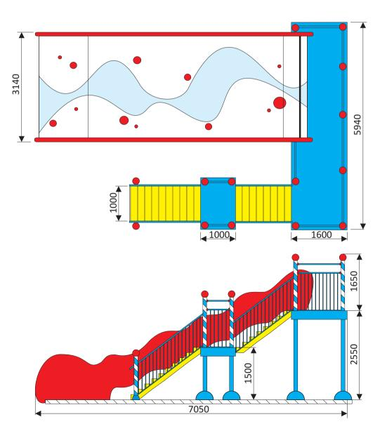
The family slide can be fixed in the pool or at the pool's surround. By fixation at the pool's edge, the water depth has to be at least 1000 mm. When the slide is placed inside the pool, the water depth can be 500 mm deep. Adjustments can be made on request.
